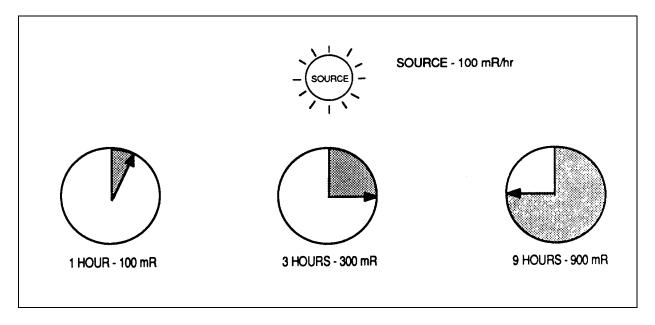
Effect of Exposure Rate and Time On Total Exposure
