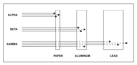
Penetrating Power of Alpha, Beta, and Gamma Radiation
