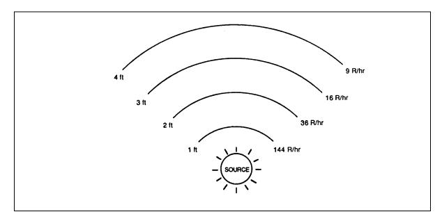
Effect of Gamma Exposure Rate and Distance On Total Exposure
