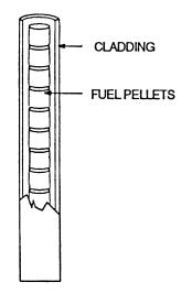
Fuel Rod With Pellets and Cladding
