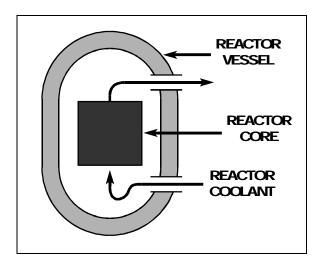
Core, Vessel, and Coolant
