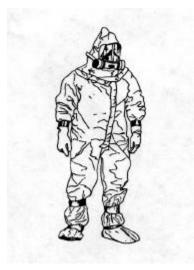
**Level C:** This level of protection can be used when proper respiratory protection can be afforded by air-purifying, canister-equipped protective breathing devices. It provides the same level of skin protection as Level B, but a lower level of respiratory protection.
