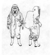
**Level A**: This level of protection should be worn when the highest level of respiratory, skin, eye, and mucous membrane protection is needed. It consists of fully encapsulating, chemical resistant clothing and self-contained breathing apparatus.
