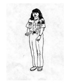
**Level D:** This protective ensemble consists primarily of a standard work uniform. It provides no respiratory protection and affords only minimal skin protection.
