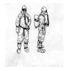
**Level B:** This level of protection should be used when the highest level of respiratory protection is required, but a lesser level of skin and eye protection is sufficient.
